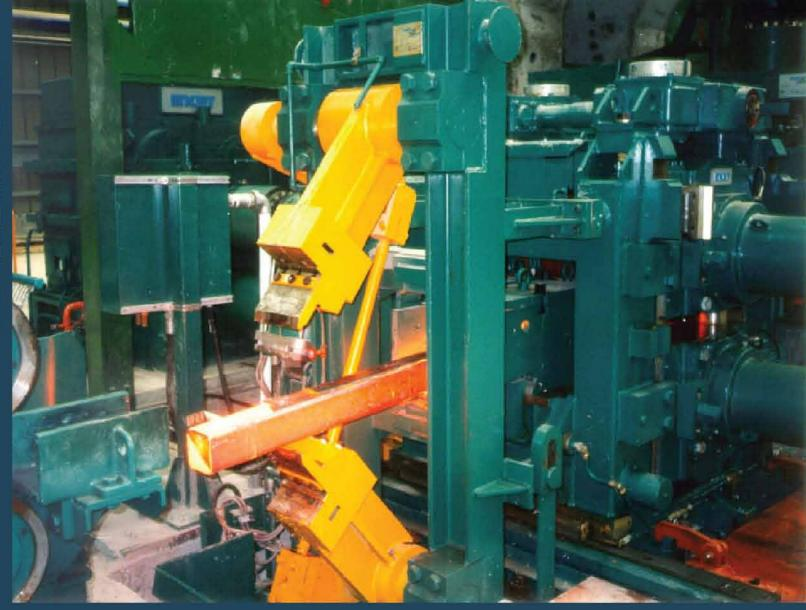
Snap shears arranged at stand #1 entry side.
